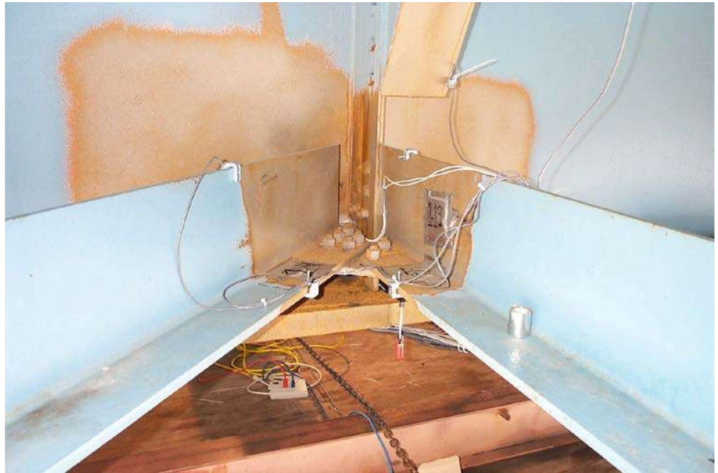
Figure 15.4.3 Strain Gage Used on the Hoan Bridge, Milwaukee, Wisconsin
