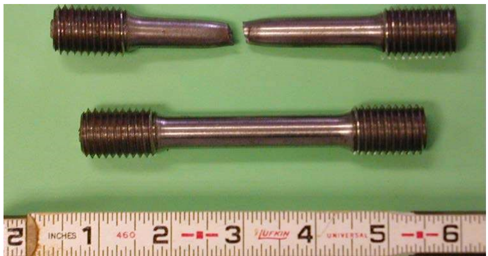
Figure 15.3.15 Ductile Failure of Cold Rolled Steel
