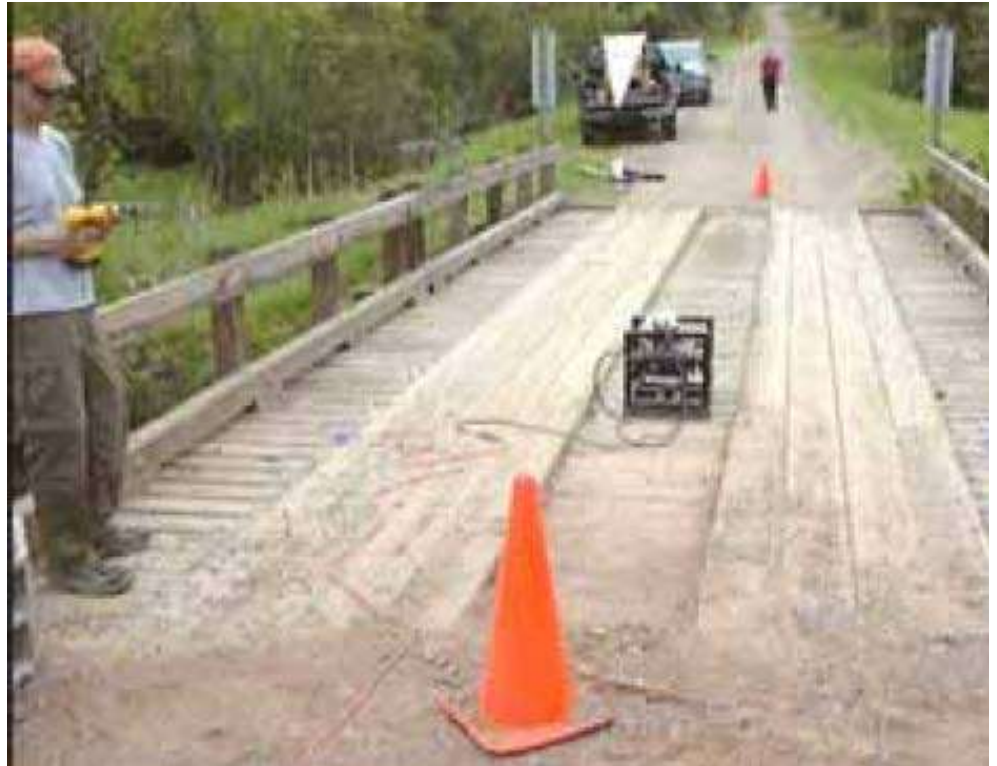
Figure 15.1.4 Vibration Testing Equipment
