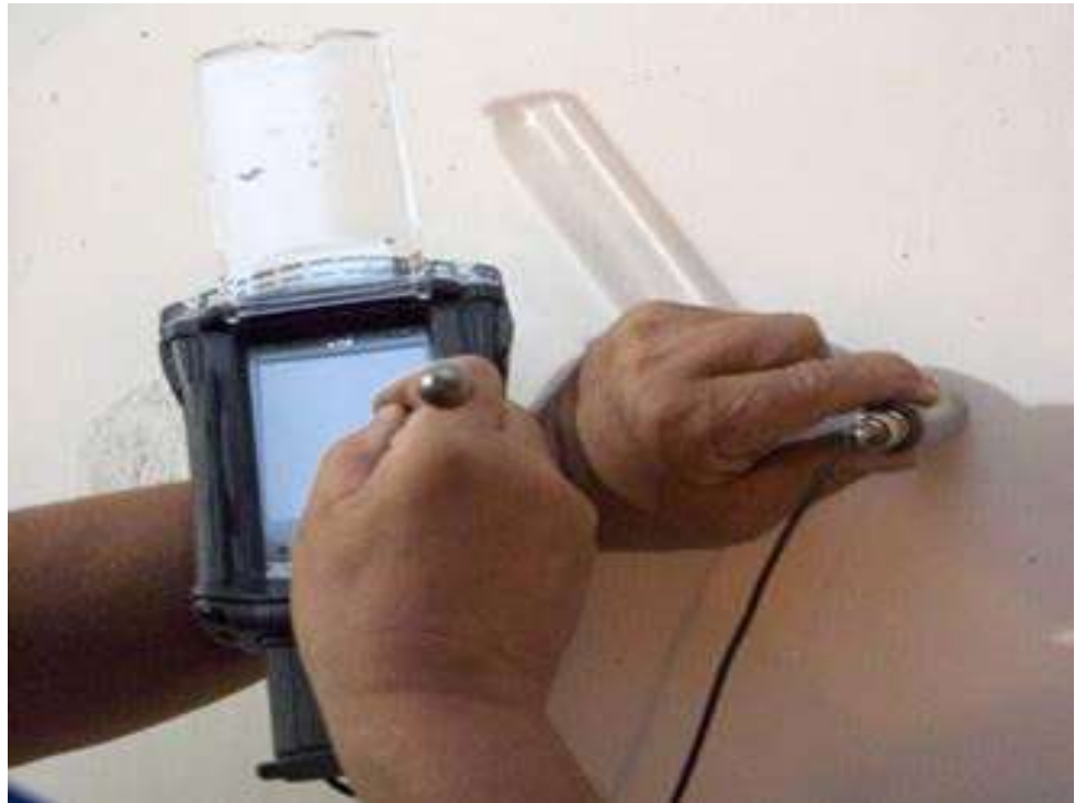
Figure 15.2.8 Impact-Echo Testing Equipment
