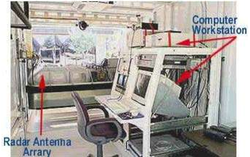
Figure 15.2.7 The HERMES Bridge Inspector (Inside)
