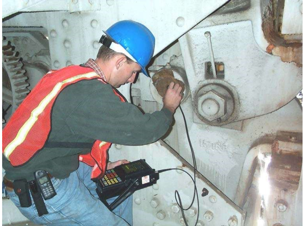
Figure 15.3.8 Ultrasonic Testing of a Pin in a Moveable Bridge
