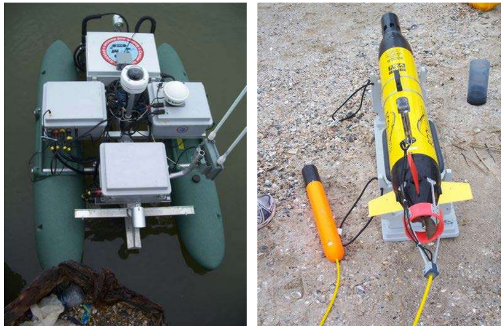
Figure 15.3.7 Robotic Inspection: Unmanned and Underwater Inspection Vehicles
