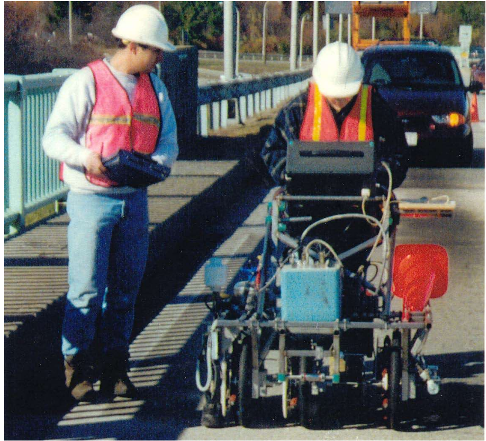
Figure 15.2.4 Delamination Detection Machinery
