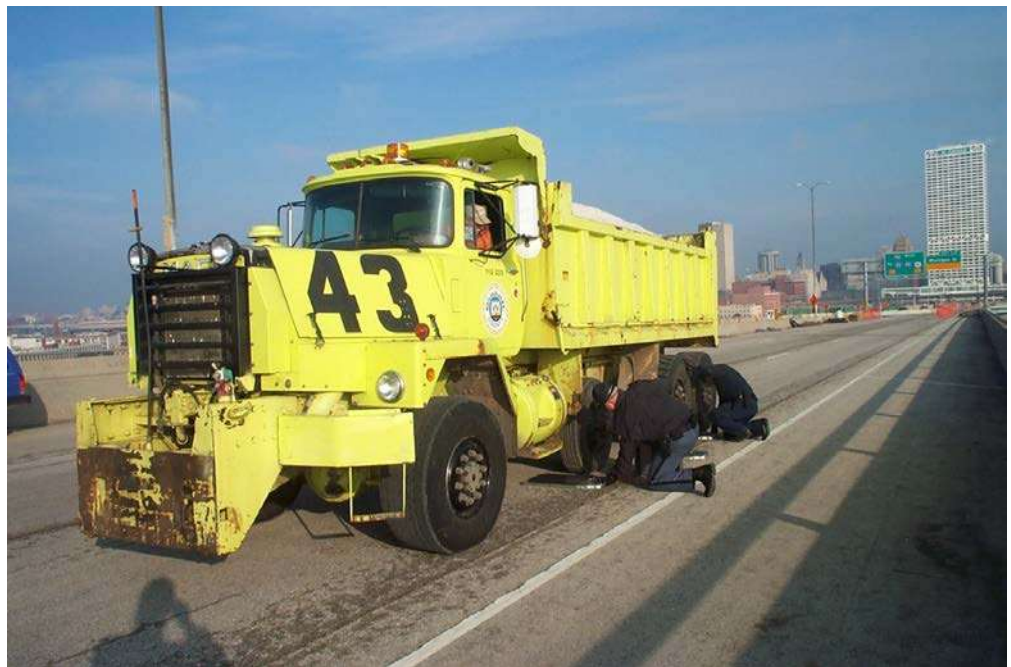
Figure 15.4.4 Dynamic Load Testing Vehicle
