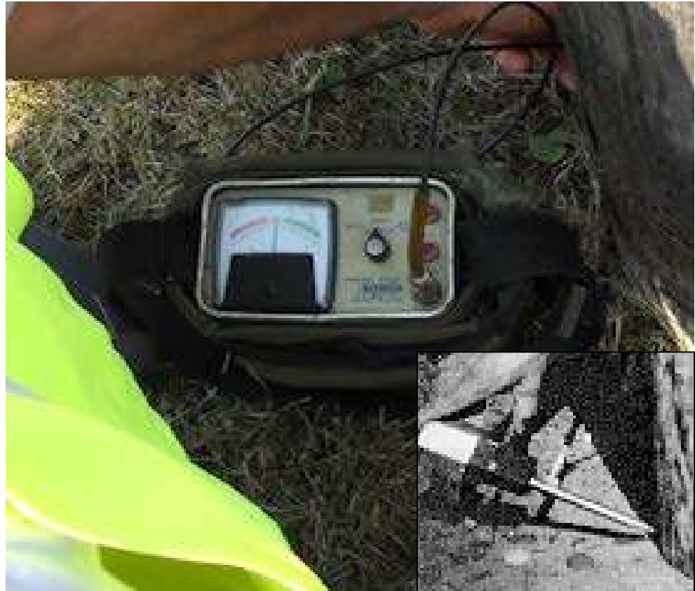
Figure 15.1.1 Sonic Testing Equipment
