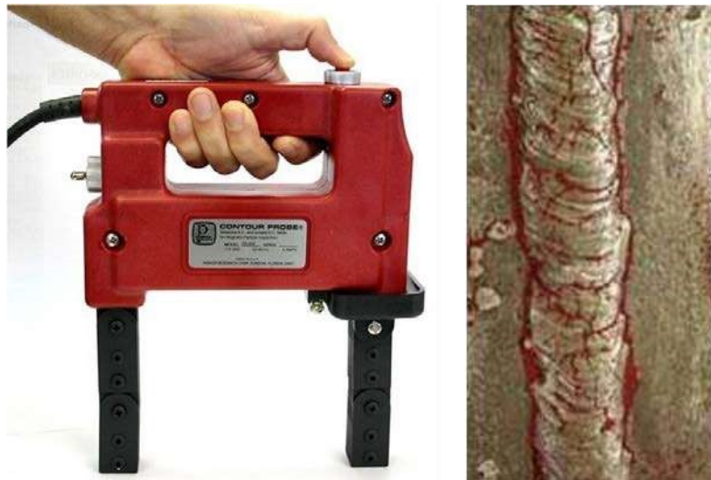
Figure 15.3.4 Magnetic Particle Device Used to Detect Subsurface Flaws
