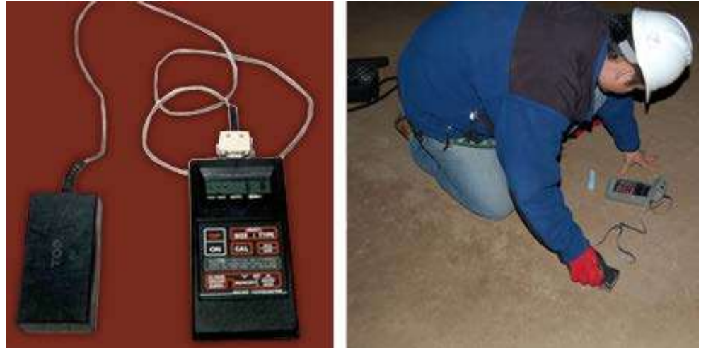
Figure 15.2.12 Pachometer Testing Equipment
